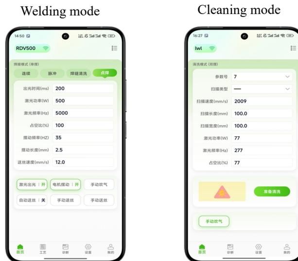
The RDWelder mobile APP supports single swing welding, single swing cleaning, double swing welding, and double swing cleaning. After connecting to the control board, the APP will automatically adapt to the current processing mode of the control card.
