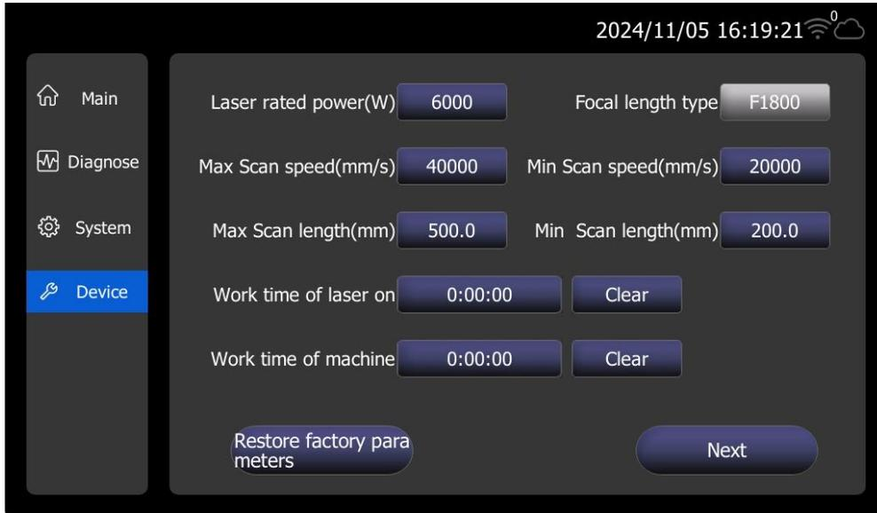
**Rated power of laser:** Used for setting the rated power of the laser.
